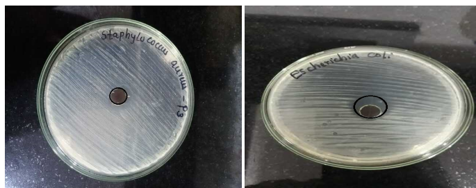
Figure 6. S. aureus and E. coli bacterial colonies cultured on petri dishes, demonstrating the antibacterial efficacy of CuO nanoparticles annealed at temperatures of 250°C and 300°C.
